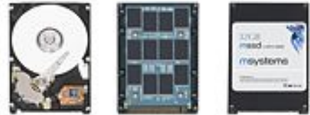
2.5" SSD (right & center) v.s. HDD (left)
