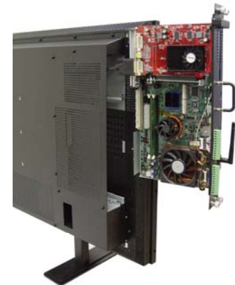
Wincomm's patented swappable drawer design
