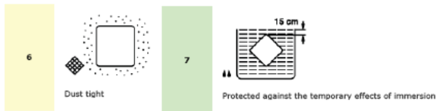
The IEC 60529 IP67 enclosure protection illustration
