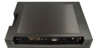
WLP-7821-17 chassis w/ aluminum plate rear cover & TV card integrated
