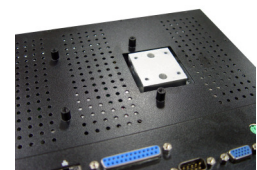
WLP-7820-10A fin-like rear plate heatsink design
