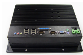
WLP-7820-10A fin-like rear plate heatsink design
