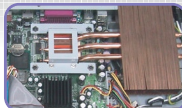
Specific Thermal Solution <40dB with P4 3.06GHz / 100% CPU loading
